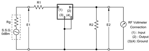
$R_g + R_1 = R_2 = \text{Input/Output Impedance}$
